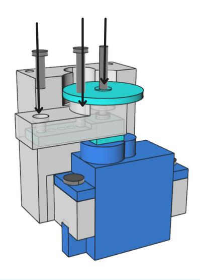
Place the servo into the servo mount
