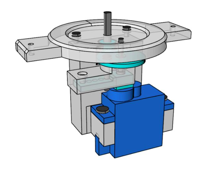
Insert the D-shaft into the D-Shaped Hole Gear and then put it into the servo mount.
