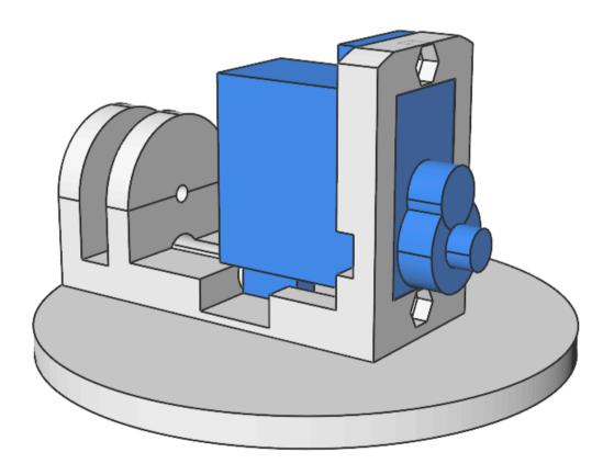
Place the servo onto the servo base
