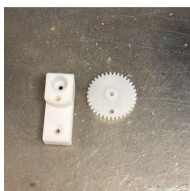
Place the gear on the table and place the horn fixture on the gear.
