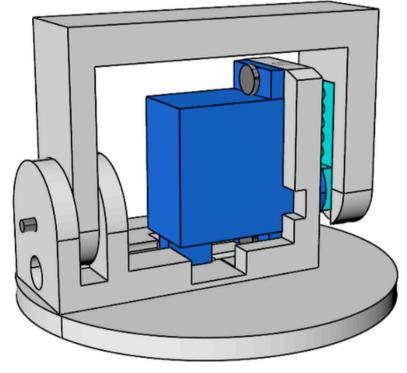
Test the servo's 0° angle before install the horn
