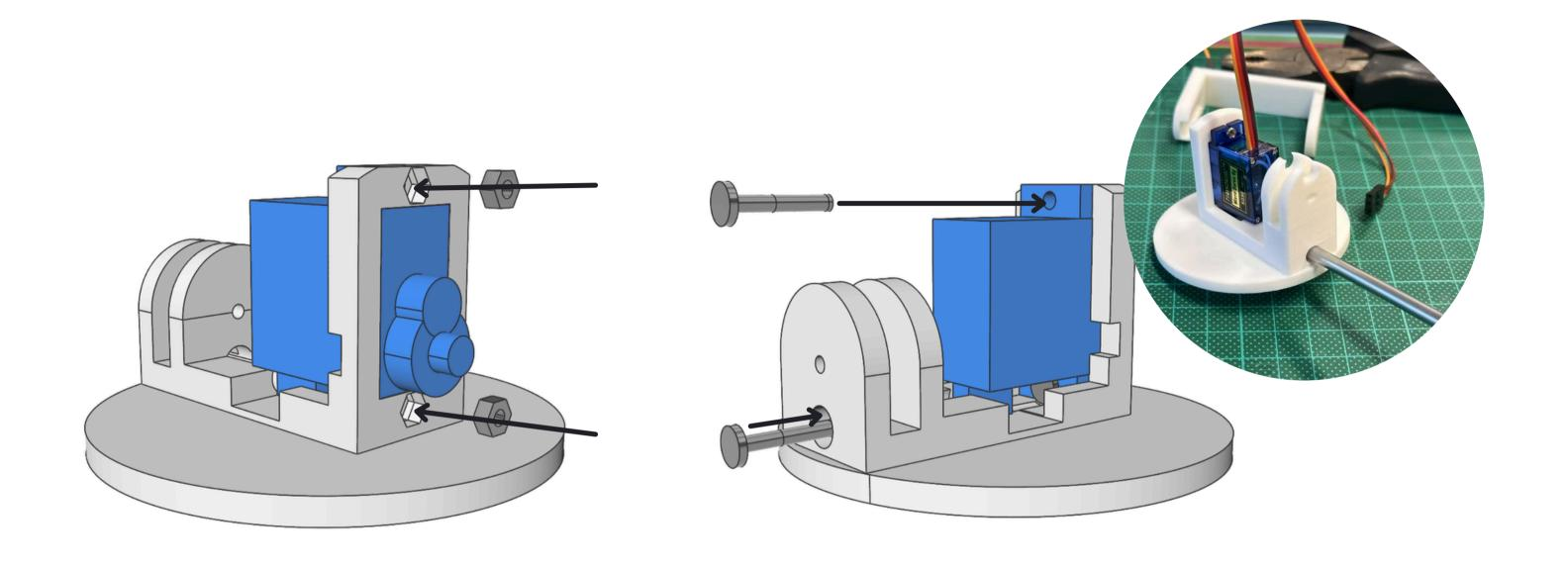
Put in the nuts and secure the servo with the bolts.
